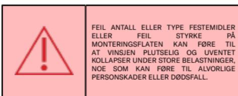
**FEIL ANTALL ELLER TYPE FESTEMIDLER ELLER FEIL STYRKE PÅ MONTERINGSFLATEN KAN FØRE TIL AT VINSJEN PLUTSELIG OG UVENTET KOLLAPSER UNDER STORE BELASTNINGER, NOE SOM KAN FØRE TIL ALVORLIGE PERSONSKADER ELLER DØDSFALL.**
