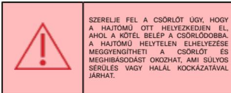
**SZERELJE FEL A CSÖRLÖT ÚGY, HOGY A HAJTOMŰ OTT HELYEZKEDJEN EL, AHOL A KÖTÉL BELEP A CSÖRLÖDOBBA. A HAJTOMŰ HELYETLEN ELHELYEZÉSE MEGGYENGÍTHETI A CSÖRLÖT ÉS MEGHIBÁSODÁST OKOZHAT, AMI SÚLYOS SÉRÜLÉS VAGY HALÁL KOCKÁZATÁVAL JÁRHAT.**
